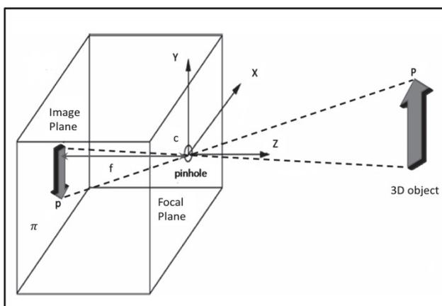
Fig. 1 The pin-hole model.
