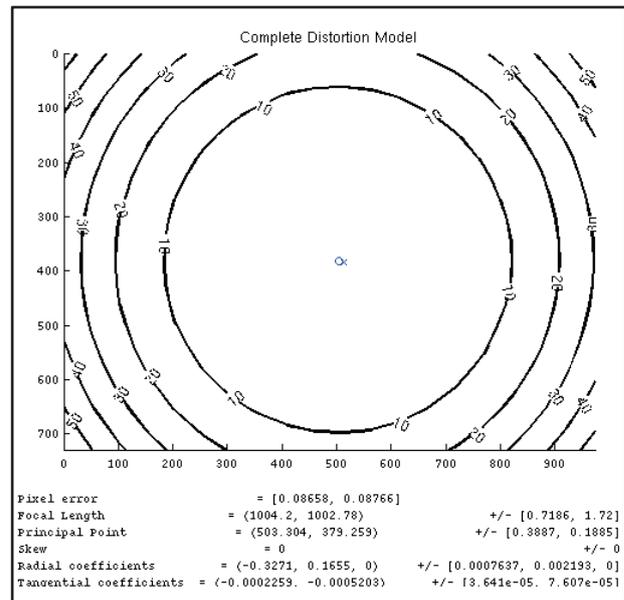
Fig. 2 Iso-distortion curves of  $D(r, t)$ .
