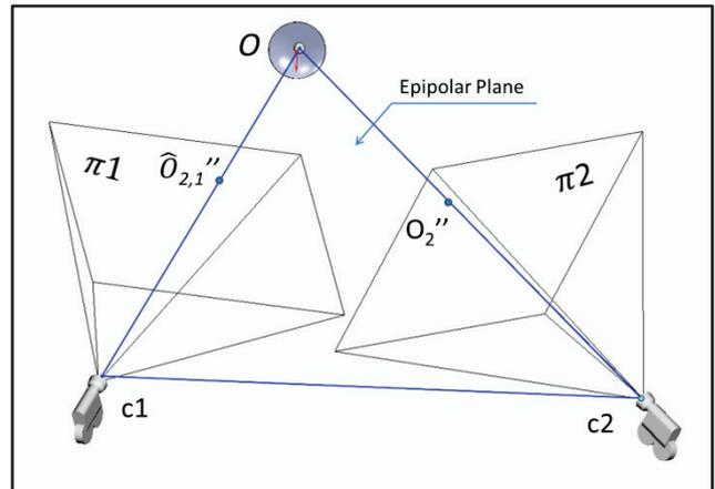
Fig. 4 Epipolar geometry.
