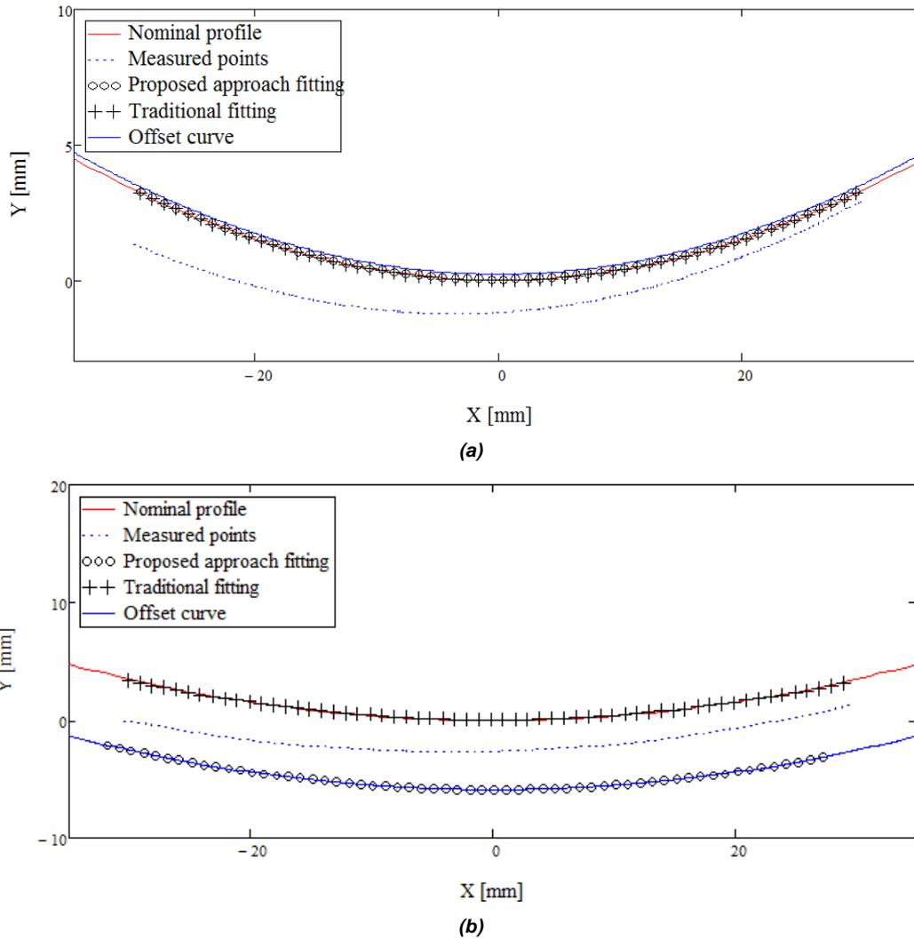
**Fig. 5 Best alignments obtained for ground mould lens (a) and polished mould lens (b)**
