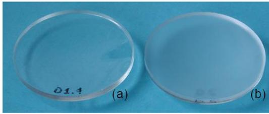
Fig. 1 Measured surfaces: (a) polished lens; (b) ground lens.
