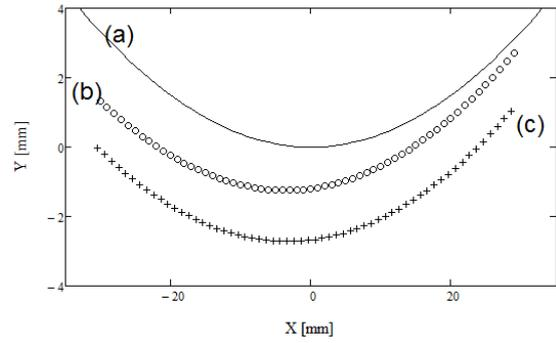
Fig. 2 Nominal profile (a),  $p$  and  $R$  are respectively  $-1.8$  and  $132.45$  mm; measured points (12000) on ground lens (b) and polished lens (c)
