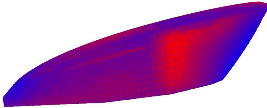
Fig. 7 Colored local deviation calculated on left lamp lens (257000 points)
