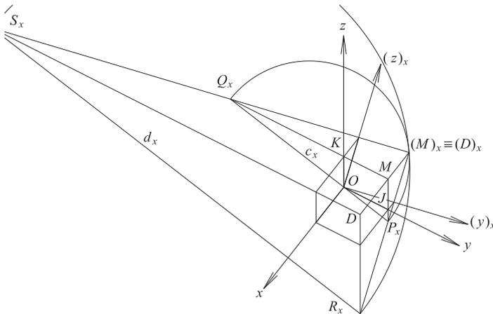
Fig. 7 Tilt of a plane perpendicular to the axis  $(z)$  on the main chart plane
