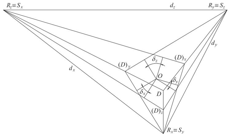
Fig. 9 Building of the axonometric perspective from the main related views
