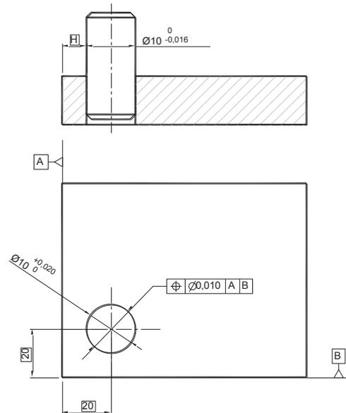
Fig. 3 Geometric specification of a functional condition.
