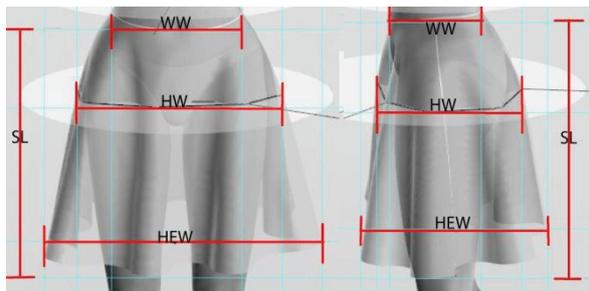
Fig. 7 Measurements Definition: 3D Simulation
